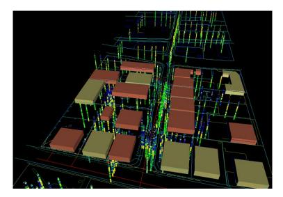
The multi-colored "straws" display subsurface geologic readings taken every one to five centimeters down to 10 meters below ground surface
